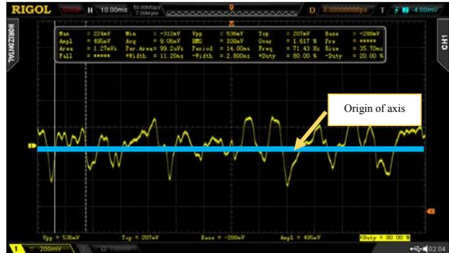
Figure 9. Output Signal of High Pass Filter Circuit
