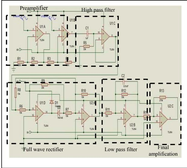
Figure 2. Complete EMG Signal Acquisition Circuit
