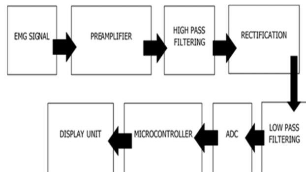
Figure 1. Overall system of EMG device
