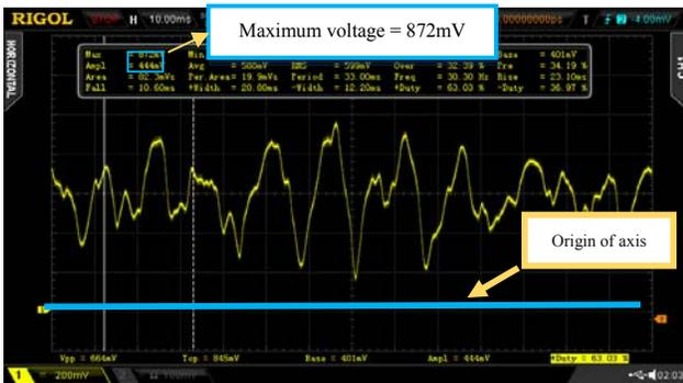
Figure 8. Output Signal of Pre-amplifier Circuit with Action
