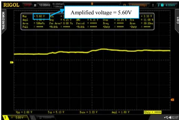
Figure 11. Output Signal after Low Pass filter and Final Amplification
