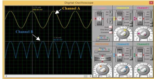
Figure 6. Simulation for Rectification Output Signal
