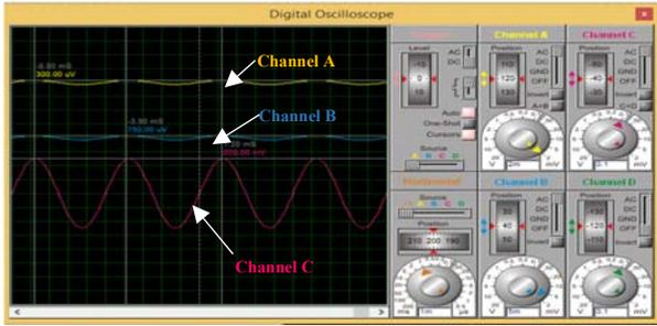
Figure 4. Simulation for Pre-amplifier Output Signal
