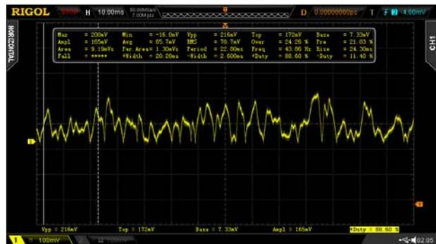
Figure 10. Output Signal of Fullwave Rectifier circuit
