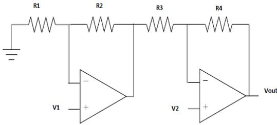
Figure 3. Two Op-Amp Instrumentation Amplifier
